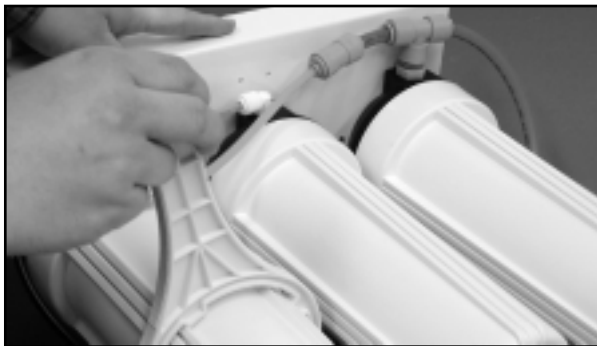
Figure 12 - Using sump wrench to change filter cartridges
