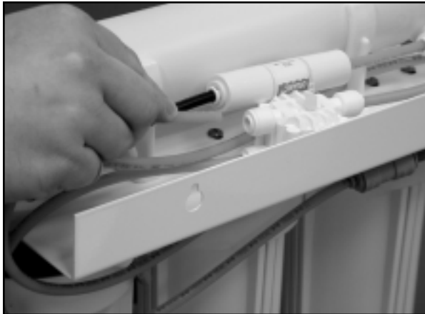
Figure 10 - Disconnect pre-carbon outlet tube from shutoff valve
