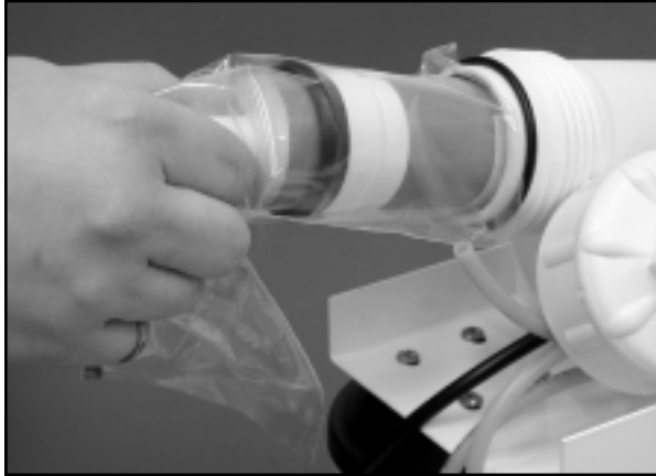
Figure 9 - Installing membrane without touching
