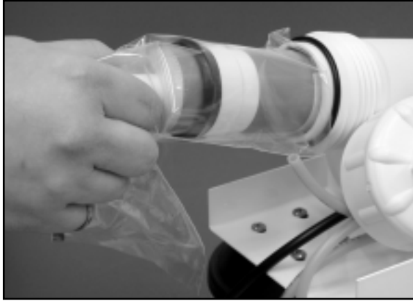
Figure 8 - Installing membrane without touching
