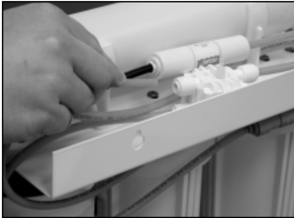
Figure 9 - Disconnect pre-carbon outlet tube from shutoff valve
