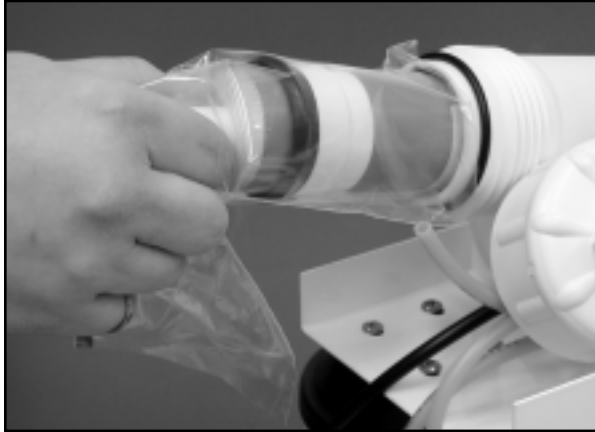
Figure 8 - Installing membrane without touching
