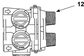
Unit 2094 includes a CPVC tank adapter - Part No. 81041
