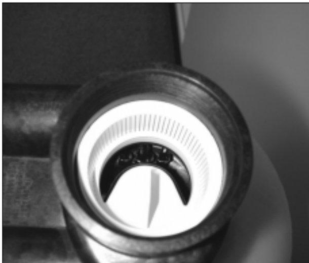
Figure 5 - The 1" In-out Head includes a removable upper distribution basket providing access to the top of the riser pipe, allowing water to be drained from the tank when replacing media.
